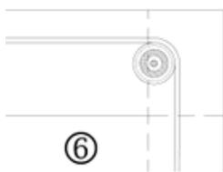
**Step 6.** The tension cord must now be run up the "U" shaped channel of the guiderail on the motor side (6). At the top of the guiderail, the tension cord must run over top of the single groove of the cord guide.
