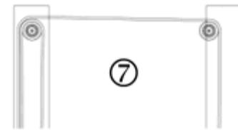
**Step 8.** The cord must now be attached to the pulley using the remaining two holes. First, you must rotate the pulley towards you ONE complete revolution. This will ensure that the cords do not cross over each other when the shutter is in operation. After rotating the pulley, fish the tension cord through the remaining slot that is furthest from you and out of the accompanying slot. Tie a double knot and tuck in any remaining "tail".
